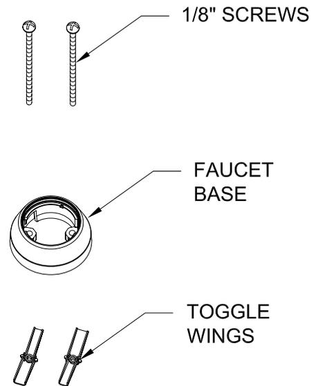
3. Assemble the 1/8" Screws & Toggle Wings into the Faucet Base. Adjust the Wings approximately 1" plus the thickness of the mounting surface away from the bottom of the Faucet Base.
